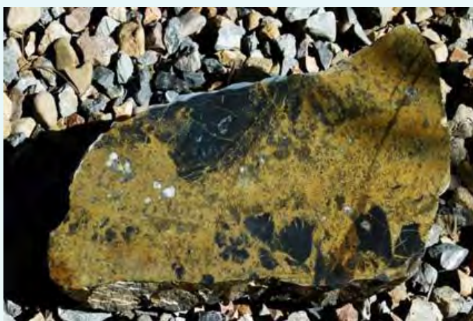
Left: Chalcopyrite with black, fractured siliceous shale or chert clasts in the 1100 Orebody at Mt Isa. Right: Detail of chalcopyrite in silica-dolomite breccia showing clearly discordant mineralisation. Both W.D. Smith specimens. Images courtesy J.R. Lord.
