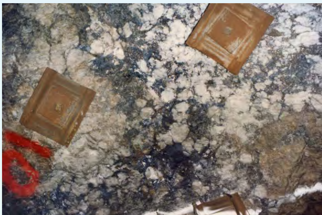
High grade Pb-Zn in brecciated quartz in the Fitzpatrick orebody at the North Mine, Broken Hill. The rectangles are plates for rock bolts. Image courtesy J.R. Lord.
